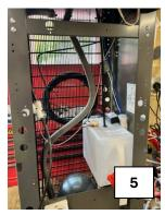
6. Empty the waste bottle through the tap on the front. It is recommended that the waste bottle is sanitised by pouring sanitising solution into the drip tray and allowing it to flow into the bottle.
