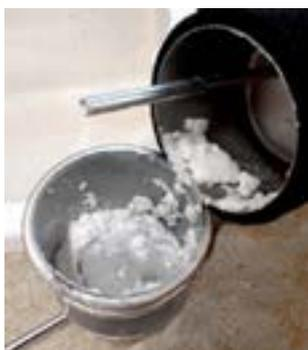
A hot tank can scale up in a relatively short time – depending on the water hardness, how hot the temperature and if there is high use.
