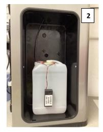
The alarm will silence once the overflow container has been emptied. Alternatively, you can switch it off manually using the switch attached to the overflow container.
