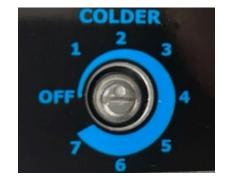
Set the thermostat on EC versions. Thermostat settings need to be adjusted through the control panel. The default settings are -2 C for the summer months and +2 C for the winter. We recommend you set both to +2C. Please see the instruction manual for programming instructions. Failure to set the thermostat correctly could lead to a frozen ice bank.
