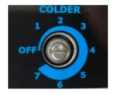
8. Set the thermostat on EC versions. Thermostat settings need to be adjusted through the control panel. The default settings are -2 C for the summer months and +2 C for the winter. We recommend you set both to +2C. Please see the instruction manual for programming instructions. Failure to set the thermostat correctly could lead to a frozen ice bank.
