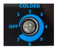
8. **Set the thermostat on EC versions.** Thermostat settings need to be adjusted through the control panel. The default settings are -2 C for the summer months and +2 C for the winter. We recommend you set both to +2C. Please see the instruction manual for programming instructions. Failure to set the thermostat correctly could lead to a frozen ice bank.
