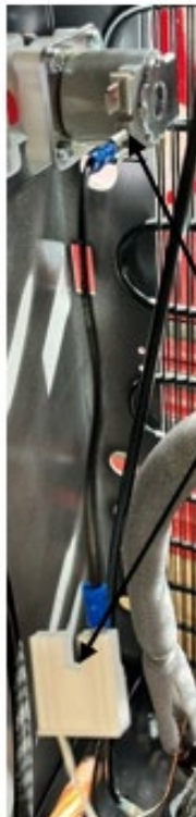
Disconnect inlet solenoid connector
