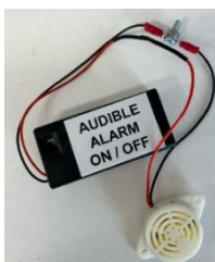
AA First Overflow Alarm
