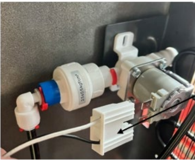
Disconnect inlet solenoid connector
